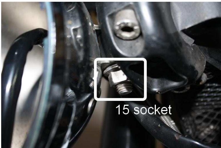
3. Use a no. 15 socket and a allen key to remove the bowl.
